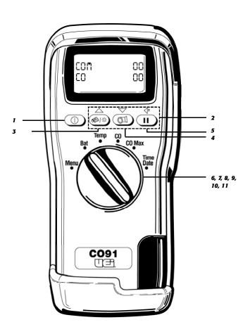
1. **Power Push-button** ①: Press " ① " button to switch the unit ON in fresh air outside the property about to be tested. This lets the meter auto calibrate its sensors properly.
