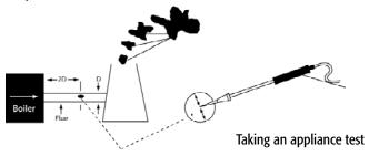
Use the probe's depth stop cone to fix it in flue diameters from 1/4 to 4/5 inch, 6 to 21 mm. Its maximum operating temperature is 1112°F / 600°C.
